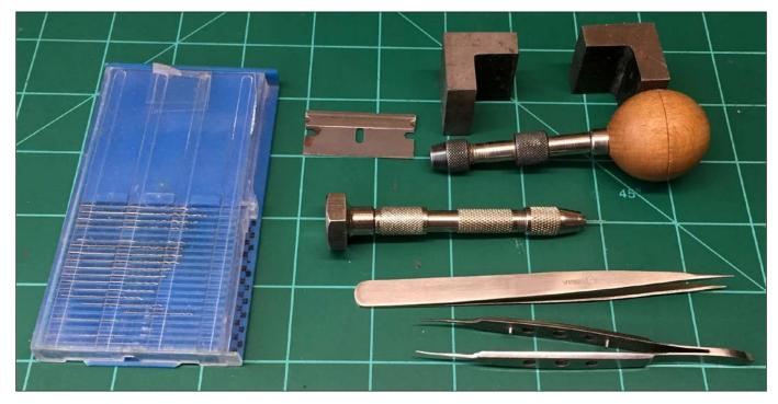
**TOOLS**: I use a single edge razor blade for 99% of my cutting work. These never roll off of the workbench, they are very light and easy to grip, and a box of 100 at Home Depot or Lowe's is inexpensive. Cutting resin does not require a new blade, especially when trimming the flash away.
