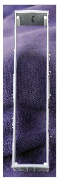
Now it's time to complete the rectangular structure. Keep the Testors<sup>®</sup> handy and a puddle of CA ready. I am left handed so I hold the structure in my right hand by one corner. After appling Testors<sup>®</sup> to the styrene, maneuver the joint until the two parts are aligned then wick in some CA. The other end will be loose. Just focus on the end you are gluing.
