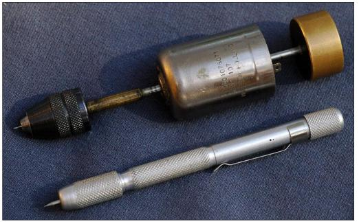
A scribe is seen below the drill and is very helpful to impress a dimple onto the resin material for the drill bit to find and stay at the point where you want a hole. A sewing needle mounted in a dowel, old pen, or pin vise makes a quick scribe that will assist in many future hobby tasks.
