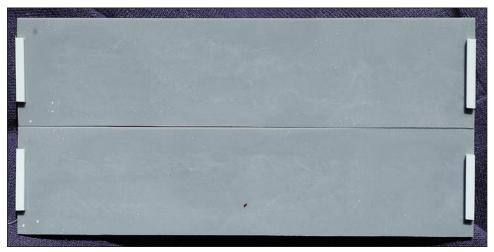
Meanwhile, I sanded the back of the end parts to thin the flash until I could flick it off with a fingernail. I have a piece of sandpaper affixed with spray adhesive to the back of a large piece of ceramic tile that is perfectly flat on its reverse side (purchased for 99 cents at Lowe's). This operation roughs up the backs of the ends to improve cement adhesion. At least that is what I tell myself.
